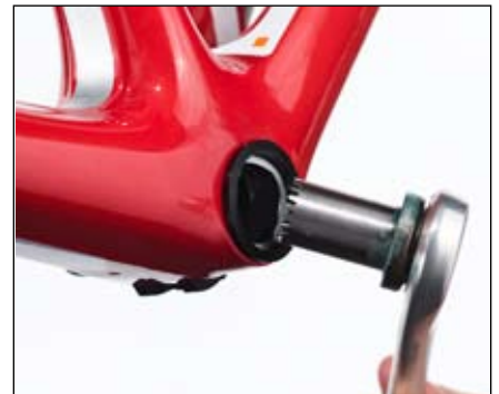
Figure 45. Inserting the non-drive side axle
